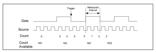
Figure 2-17. Single Triggered Pulse Width Generation Measurement
